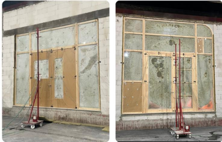
Having successfully tested two of our largest timber profiles to date, we can now provide you with a new range of tested timber door solutions that meet an EI30 fire rating with Pyroguard Protect.
