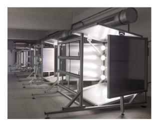
Pyroguard Protect, our toughened fire safety glass has been put under the spotlight, revealing exceptional UV durability providing results that outperform the requirements in Test Standards EN 12543 and EN 14449.
