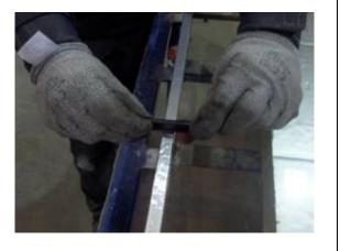
The PAL tape is then pressed onto the top face of the unit using the plastic smoothing tool.
