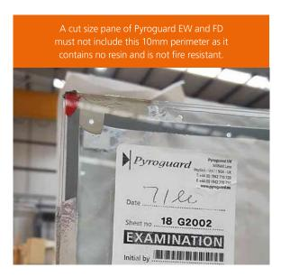
Pyrostem, 7mm Pyroguard EW and FD60 can be cut on a laminated glass cutting table or by scoring the glass by hand on each side and then snapping through. In some climatic conditions the resin layer may need the application of additional heat to separate to cut.
