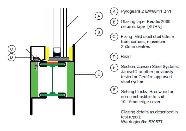
This Certificate of Approval relates to the sizes of Pyroguard Advance 2-EW60/11-2 [IGU] glass shown in Table below, when used in conjunction with the glazing system detailed previously.
