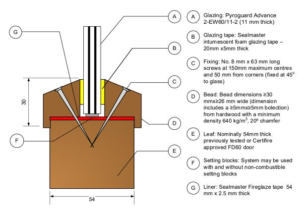
This Certificate of Approval relates to the sizes of Pyroguard Advance 2 EW60/11-2 glass shown in diagram below, when used in conjunction with the glazing system detailed previously
