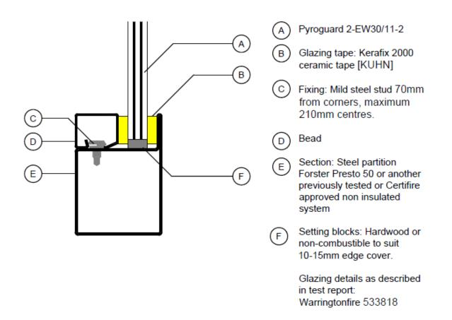
This Certificate of Approval relates to the sizes of Pyroguard Advance 2-EW30/11-2 glass shown in table below, when used in conjunction with the above system. The aspect ratio of the glass may be unlimited within these aperture dimensions.
