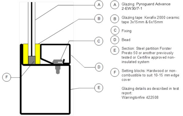
This Certificate of Approval relates to the sizes of Pyroguard Advance 2-EW30/7-1 glass shown in the table below, when used in conjunction with the above system. The maximum permitted overall screen dimensions are 3000mm high by unlimited width. The aspect ratio of the glass may be unlimited within these aperture dimensions.
