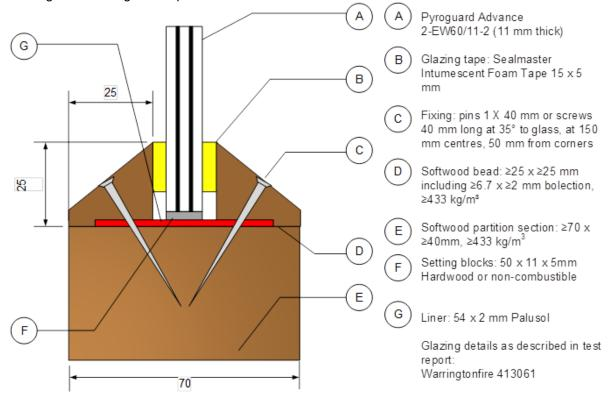
This Certificate of Approval relates to the sizes of Pyroguard Advance 2-EW60/11-2 glass shown in the table below, when used in conjunction with the above system. The aspect ratio of the glass may be unlimited within these aperture dimensions.
