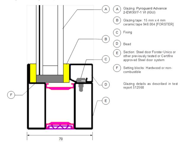
This Certificate of Approval relates to the sizes of Pyroguard Advance 2-EW30/7-1 VI [IGU] glass shown in Table below, when used in conjunction with the glazing system detailed previously.
