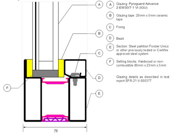
This Certificate of Approval relates to the sizes of Pyroguard Advance 2-EW30/7-1 VI glass shown in table below, when used in conjunction with the above system. The aspect ratio of the glass may be unlimited within these aperture dimensions.
