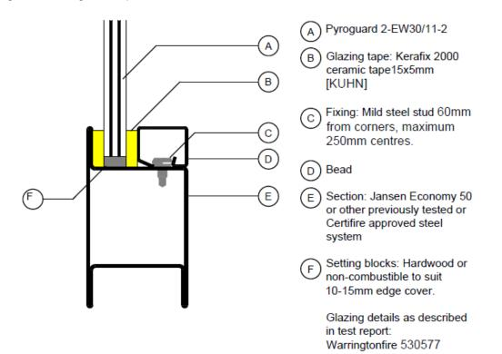
This Certificate of Approval relates to the sizes of Pyroguard Advance 2-EW30/11-2 glass shown in Table below, when used in conjunction with the glazing system detailed previously.
