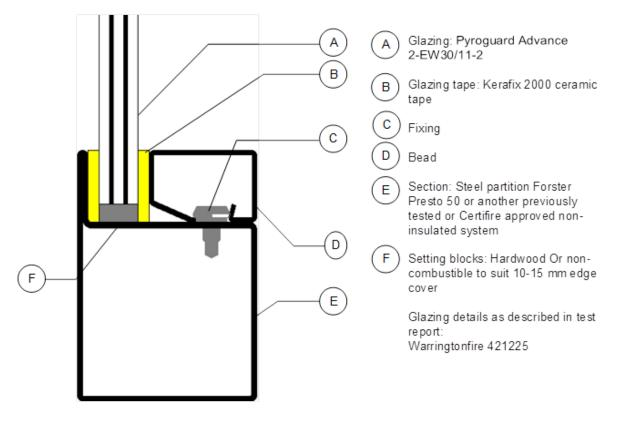
This Certificate of Approval relates to the sizes of Pyroguard Advance 2-EW30/11-2 glass shown in table below, when used in conjunction with the above system. The aspect ratio of the glass may be unlimited within these aperture dimensions.
