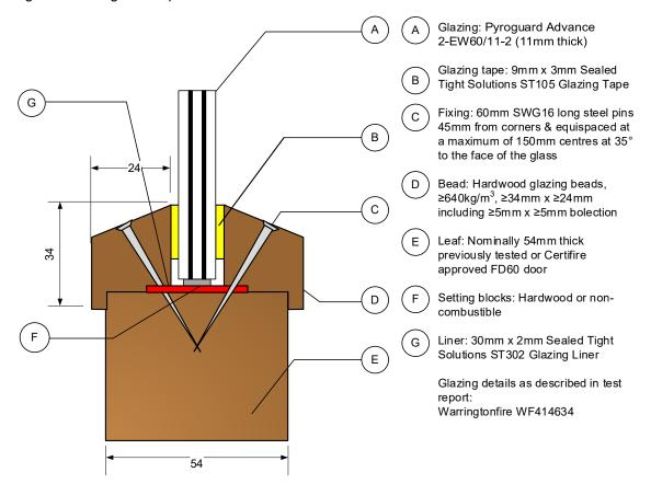
The doorset shall be CERTIFIRE approved or have test evidence for the inclusion of apertures of the proposed dimensions.
