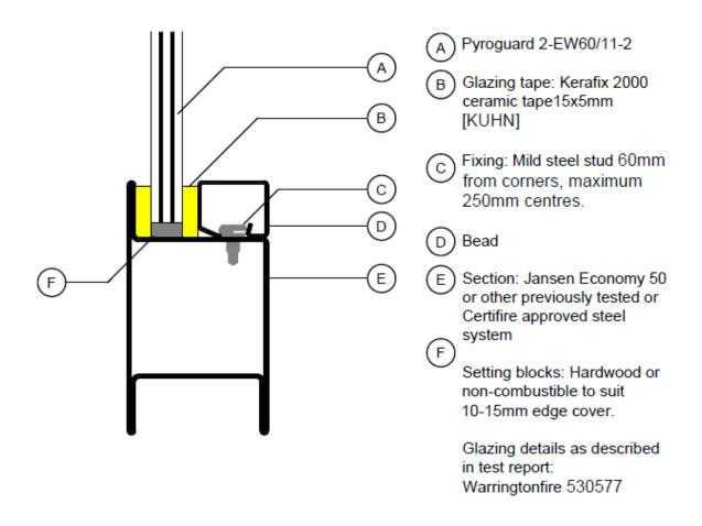
This Certificate of Approval relates to the sizes of Pyroguard Advance 2-EW60/11-2 glass shown in Table below, when used in conjunction with the glazing system detailed previously.
