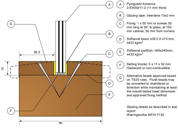
This Certificate of Approval relates to the sizes of Pyroguard Advance 2-EW30/11-2 glass shown in the table below, when used in conjunction with the above system. The aspect ratio of the glass may be unlimited within these aperture dimensions.
