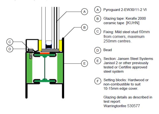
This Certificate of Approval relates to the sizes of Pyroguard Advance 2-EW30/11-2 [IGU] glass shown in Table below, when used in conjunction with the glazing system detailed previously.
