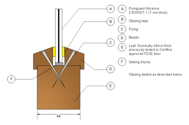
The doorset shall be CERTIFIRE approved or have test evidence for the inclusion of apertures of the proposed dimensions. This Certificate of Approval relates to the sizes of Pyroguard Advance 2-EW30/7-1 glass shown in the Table below, when used in conjunction with the above system. The aspect ratio of the glass may be unlimited within these aperture dimensions.
