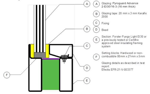
This Certificate of Approval relates to the sizes of Pyroguard Advance 2-EW30/16-3 glass shown in table below, when used in conjunction with the above system. The aspect ratio of the glass may be unlimited within these aperture dimensions.
