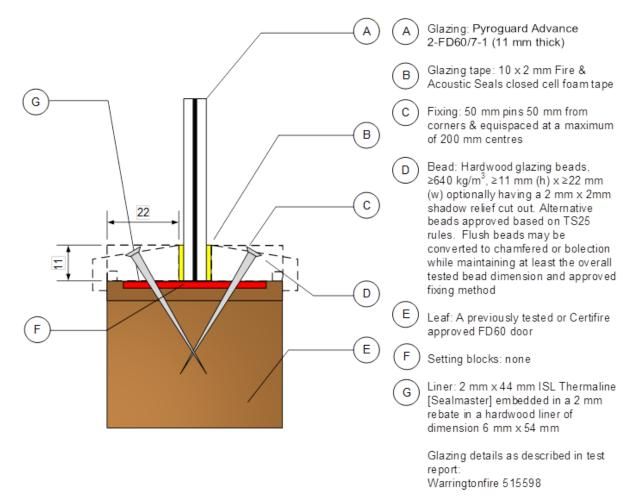
This Certificate of Approval relates to the sizes of Pyroguard Advance 2-FD60/11-1 glass shown in Table below, when used in conjunction with the glazing system detailed previously.
