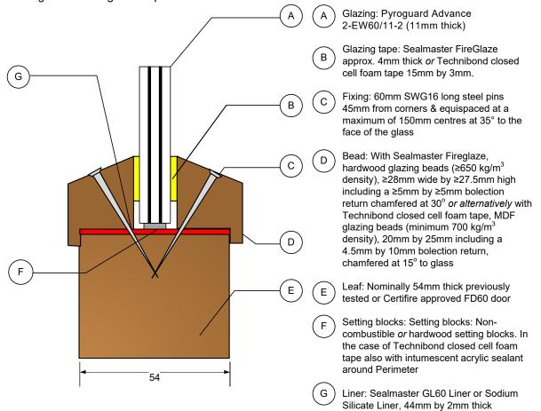
The doorset shall be CERTIFIRE approved or have test evidence for the inclusion of apertures of the proposed dimensions.
