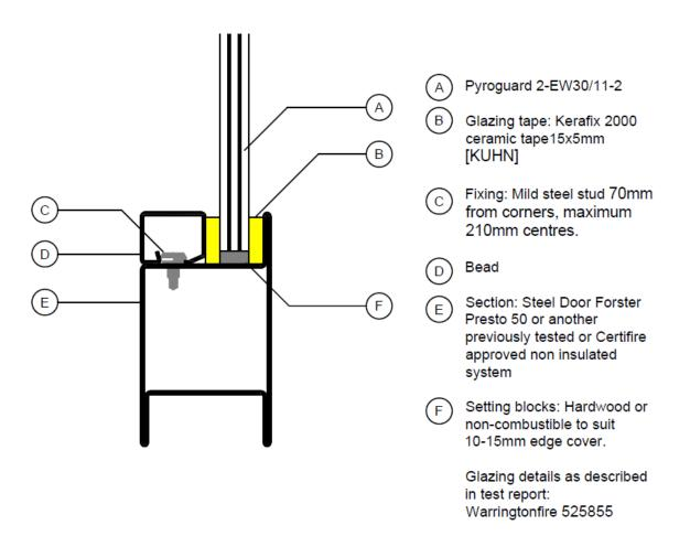
This Certificate of Approval relates to the sizes of Pyroguard Advance 2-EW30/11-2 glass shown in Table below, when used in conjunction with the glazing system detailed previously.
