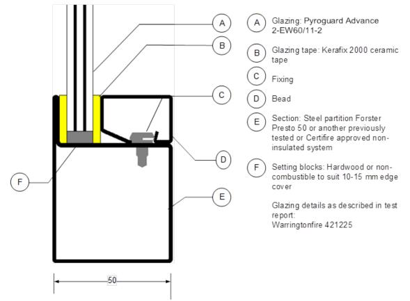
This Certificate of Approval relates to the sizes of Pyroguard Advance 2-EW60/11-2 glass shown in table below, when used in conjunction with the above system. The aspect ratio of the glass may be unlimited within these aperture dimensions.
