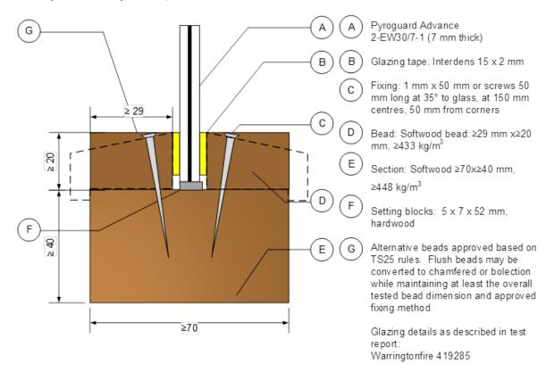
This Certificate of Approval relates to the sizes of Pyroguard Advance 2-EW30/7-1 glass shown in the table below, when used in conjunction with the above system. The aspect ratio of the glass may be unlimited within these aperture dimensions.
