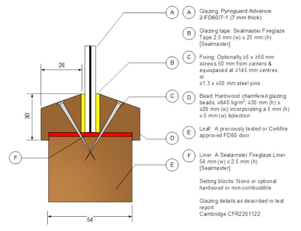
This Certificate of Approval relates to the sizes of Pyroguard Advance 2-FD60/7-1 glass shown in Table below, when used in conjunction with the glazing system detailed previously.
