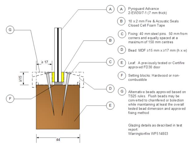
This Certificate of Approval relates to the sizes of Pyroguard Advance 2-EW30/7-1 glass shown in the table below, when used in conjunction with the above system. The aspect ratio of the glass may be unlimited within these aperture dimensions.
