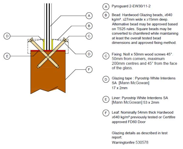
This Certificate of Approval relates to the sizes of Pyroguard Advance 2-EW30/11-2 glass shown in the table below, when used in conjunction with the above system. The aspect ratio of the glass may be unlimited within these aperture dimensions.
