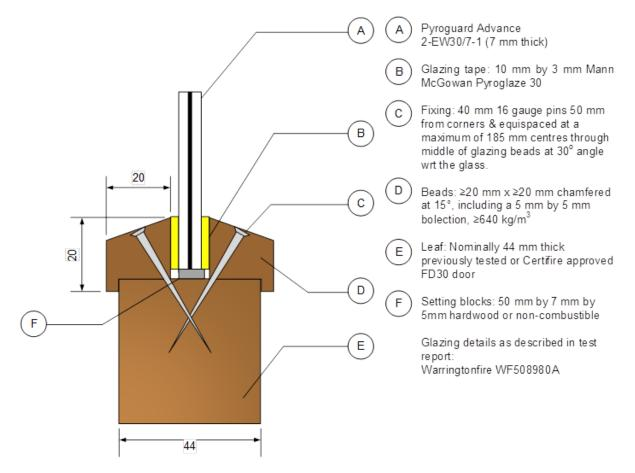
This Certificate of Approval relates to the sizes of Pyroguard Advance 2-EW30/7-1 glass shown in the table below, when used in conjunction with the above system. The aspect ratio of the glass may be unlimited within these aperture dimensions.
