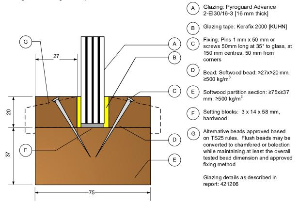
This Certificate of Approval relates to the sizes of Pyroguard Advance 2-EI30/16-3 glass shown in the table below, when used in conjunction with the above system. The aspect ratio of the glass may be unlimited within these aperture dimensions.
