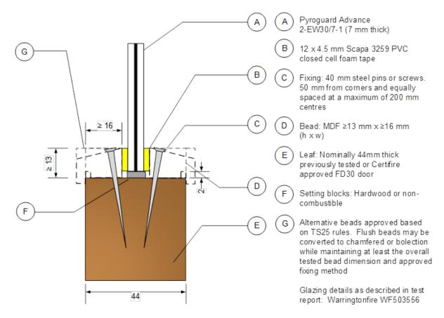
This Certificate of Approval relates to the sizes of Pyroguard Advance 2-EW30/7-1 glass shown in the table below, when used in conjunction with the above system. The aspect ratio of the glass may be unlimited within these aperture dimensions.
