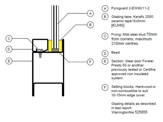
This Certificate of Approval relates to the sizes of Pyroguard Advance 2-EW90/11-2 glass shown in Table below, when used in conjunction with the glazing system detailed previously.
