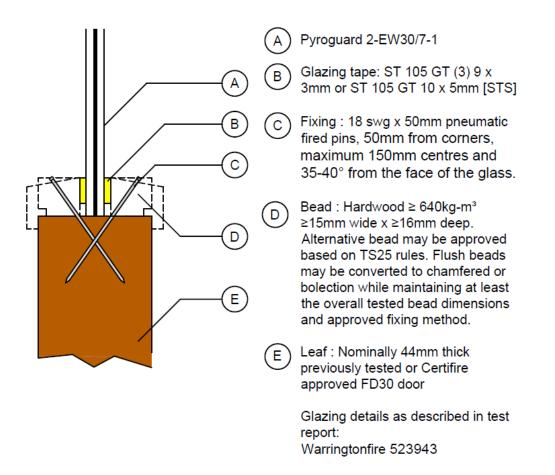
This Certificate of Approval relates to the sizes of Pyroguard Advance 2-EW30/7-1 glass shown in the table below, when used in conjunction with the above system. The aspect ratio of the glass may be unlimited within these aperture dimensions.
