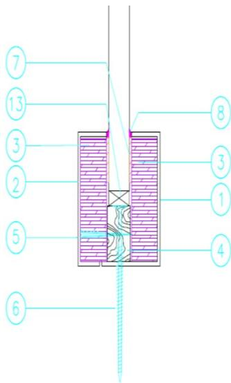
1. 60 mm wide by 43 mm deep by 2 mm thick, steel screen framing
